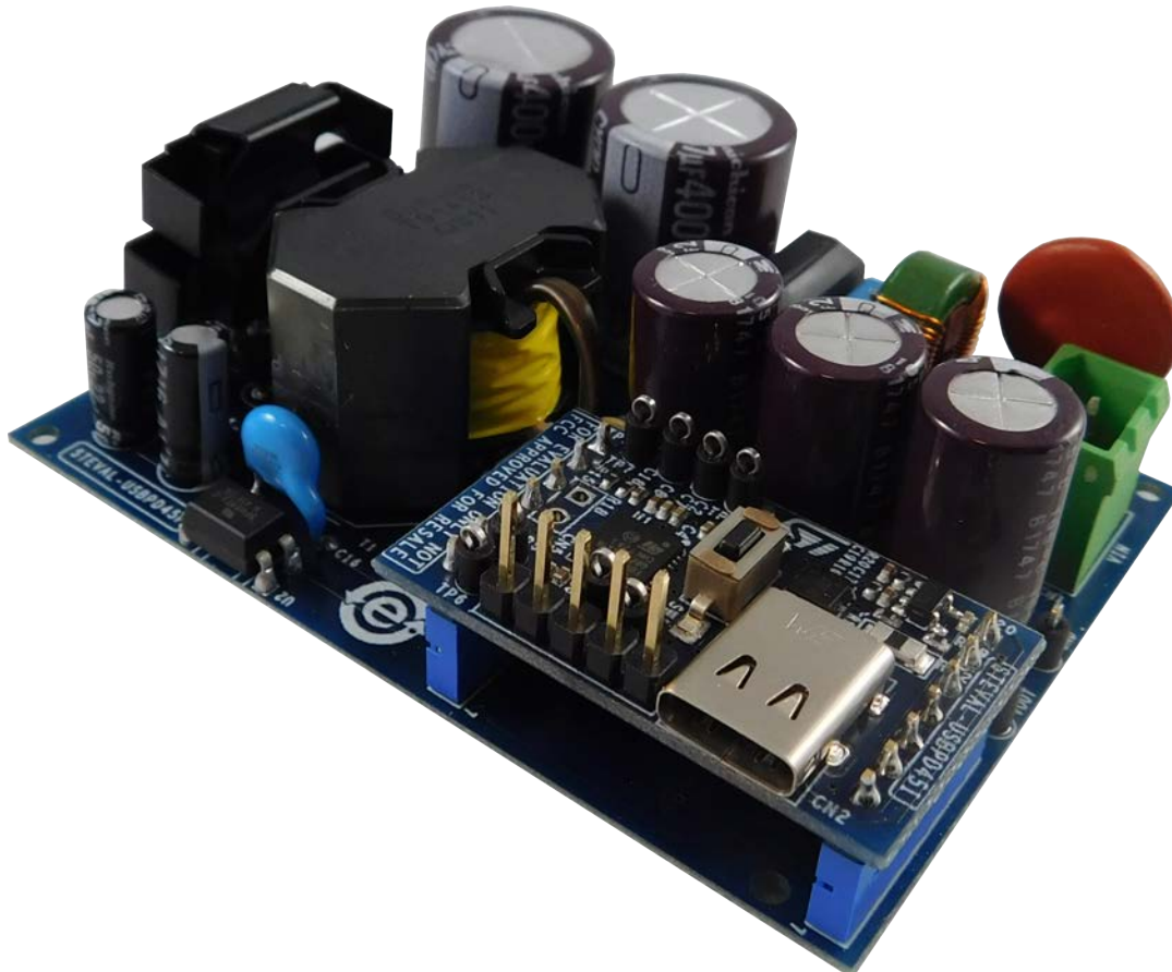
Figure 1. STEVAL-USBPD45C reference design
