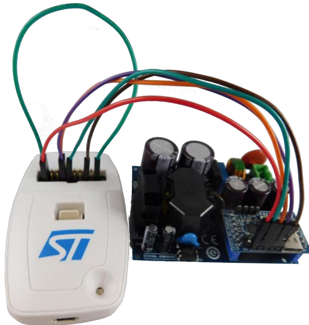
Figure 24. Setup to program the reference design with ST-LINK/V2
