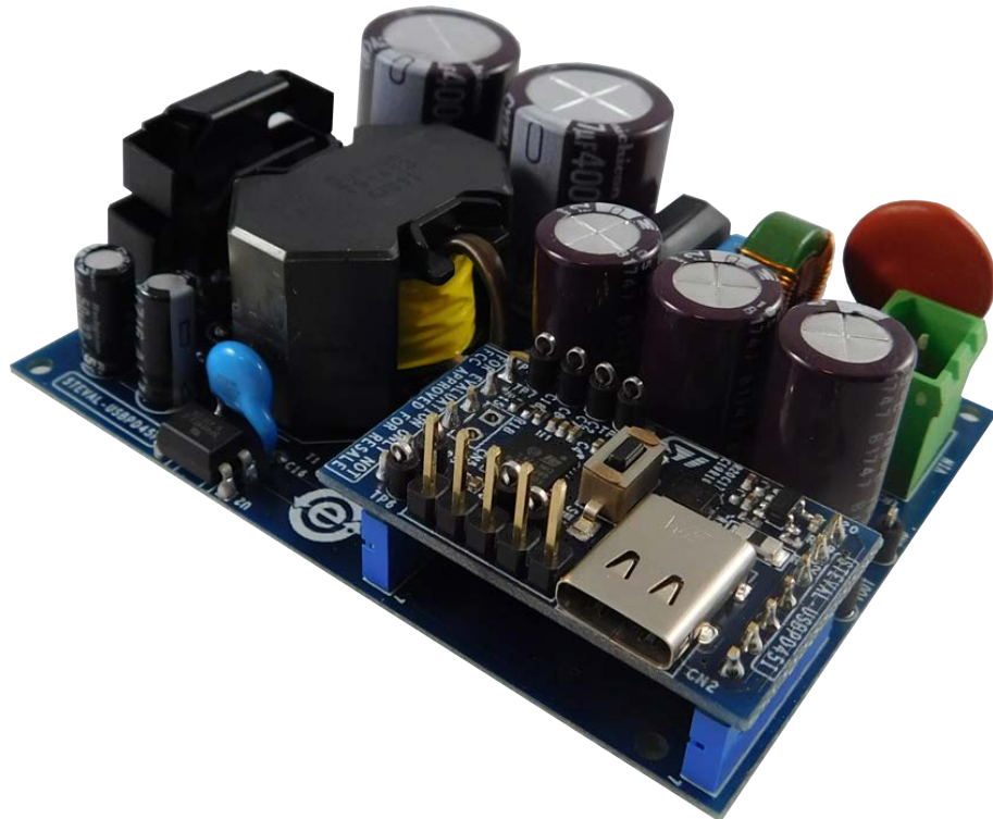
Figure 22. Orientation for stacking the digital control board on the power supply board
