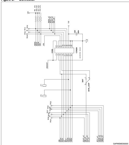
Figure 4. JTAG adapter (separated PCB)
