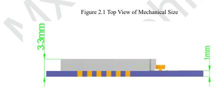
Figure 2.2 Side View of Mechanical Size
