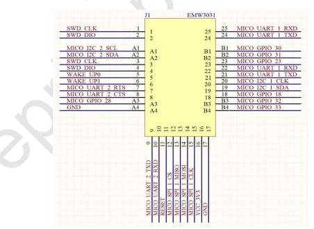
Figure 2.8 Wi-Fi Circuit
