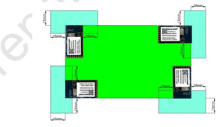
Figure 2.11 Position of the Module
