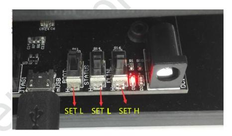
Figure 3.1 Switches of the develop board
