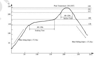
Figure 4.2 Temperature Curve of Secondary Reflow
