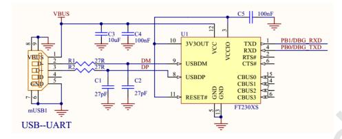
Figure 2.6 Conversion Circuit of USB to Serial Port Debugging
