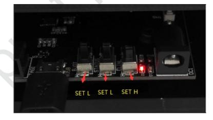
Figure 3.8 Switch Set Up at Testing Mode
