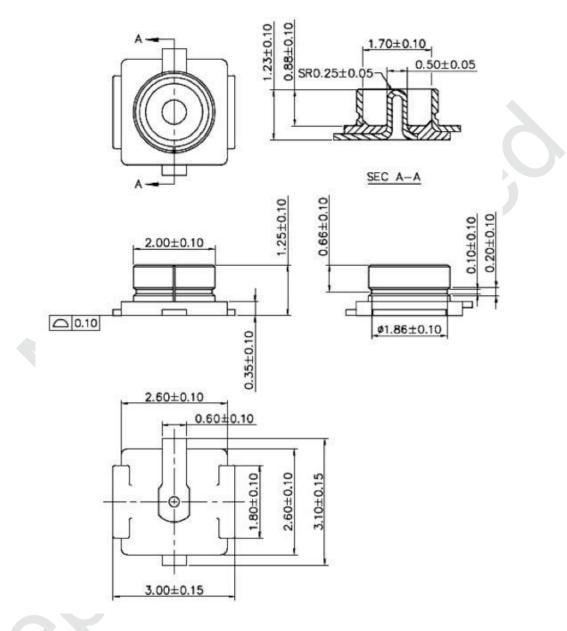
Figure 2.12 Size of External Antenna
