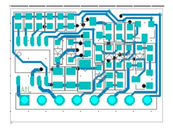
Figure 6, Bottom View of PWM control board's PCB
