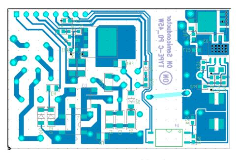
Figure 4, Bottom View of Mainboard's PCB
