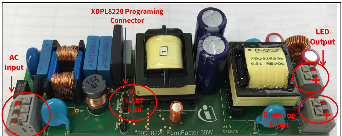
Figure 1 XDPL8220 50W reference design with isolated dimming interface and configuration connector
