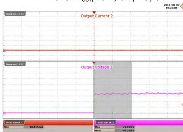
Figure 131 – 100 VAC, 60 V LED Load. Open Load_2 Start-up. Upper: I OUT , 100 mA / div. Lower: V OUT , 20 V / div., 4 s / div.
