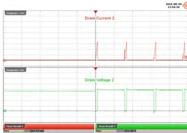
Figure 107 – 300 VAC, 52 V LED Load. Upper: I_{DRAIN} , 200 mA / div. Lower: V_{DRAIN} , 100 V / div., 4 \mu s / div.
