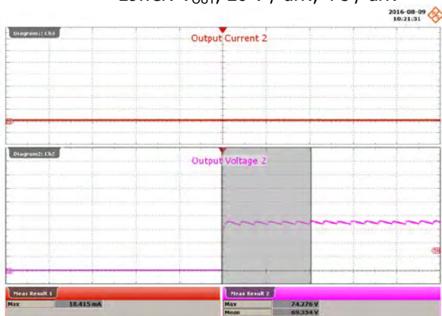
Figure 130 – 100 VAC, 60 V LED Load. Open Load_2 Start-up. Upper: I OUT , 100 mA / div. Lower: V OUT , 20 V / div., 4 s / div.
