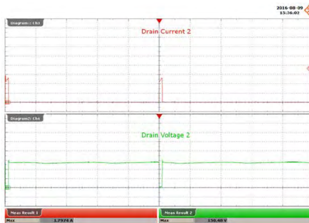
Figure 113 – 100 VAC, Output Short-Circuit. Upper: I_{DRAIN} , 500 mA / div. Lower: V_{DRAIN} , 50 V / div., 4 \mu s / div.
