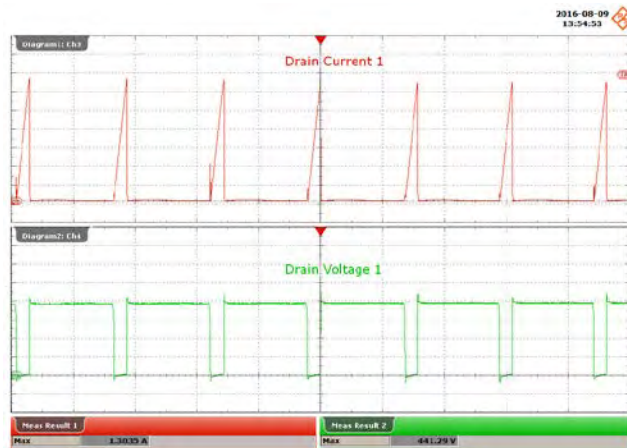
Figure 91 – 300 VAC, 52 V LED Load. Upper: I_{DRAIN} , 200 mA / div. Lower: V_{DRAIN} , 100 V / div., 10 \mu s / div.
