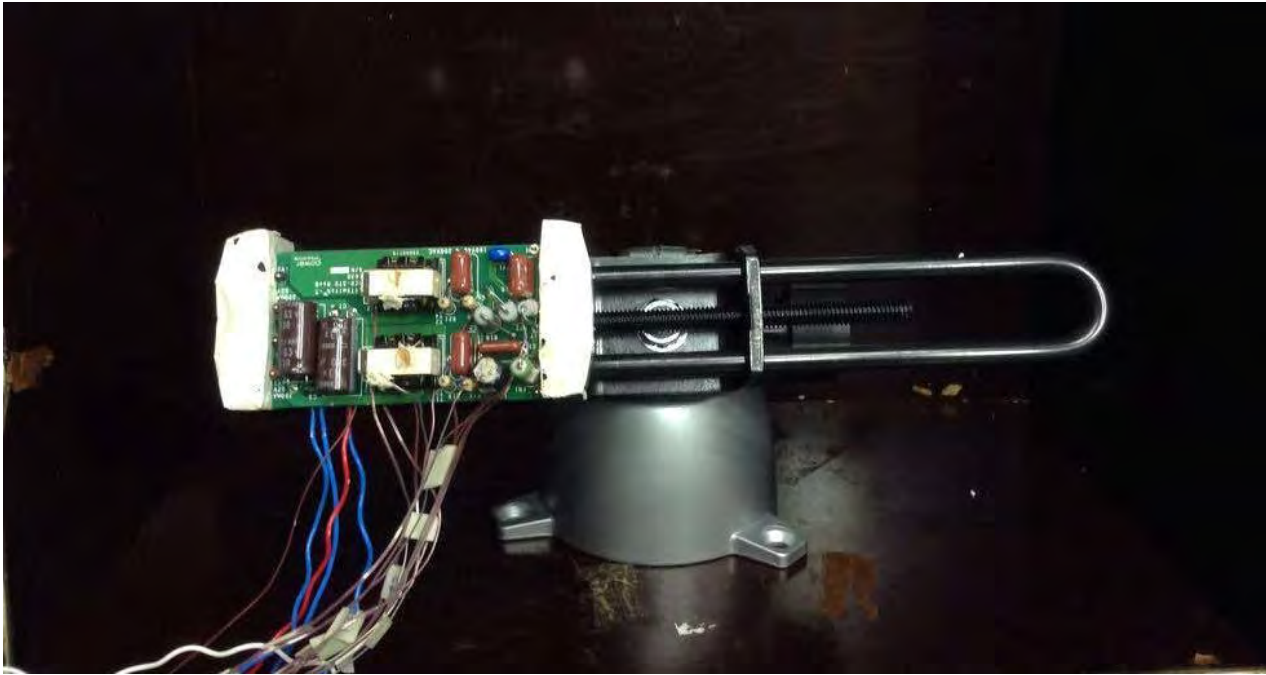
Figure 55 – Test Set-up Picture Thermal at 60 °C Ambient - Open Frame.
