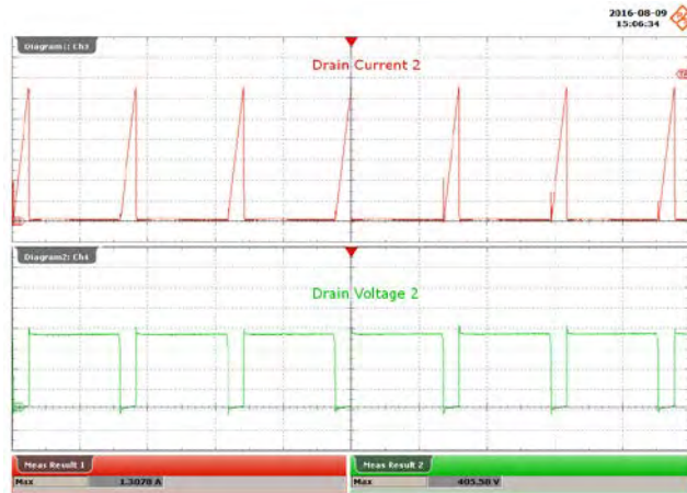
Figure 97 – 277 VAC, 52 V LED Load. Upper: I_{DRAIN} , 200 mA / div. Lower: V_{DRAIN} , 100 V / div., 10 \mu s / div.
