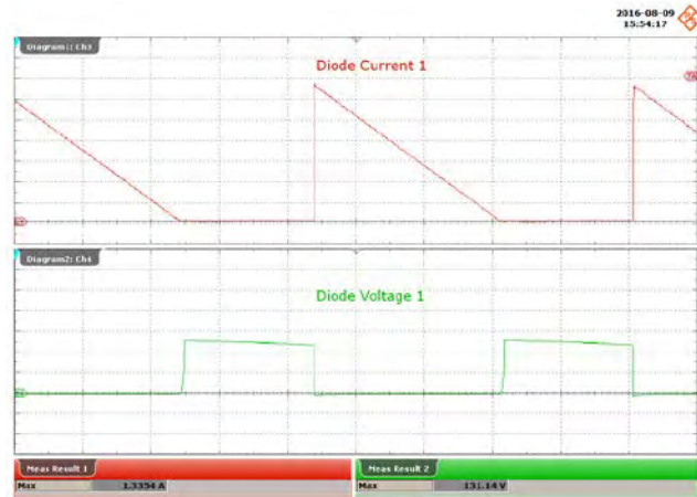
Figure 121 – 100 VAC, 52 V LED Load. Upper: I_{D1} , 200 mA / div. Lower: V_{D1} , 50 V / div., 5 \mu s / div.
