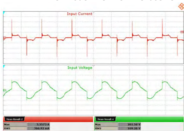
Figure 66 – 120 VAC, 52 V LED Loads. Maximum (132°) Conduction Angle. Upper: I_{IN} , 1 A / div. Lower: V_{IN} , 100 V / div., 10 ms / div.
