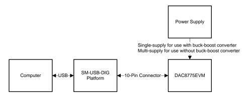
Figure 1. DAC8775EVM Hardware Setup
