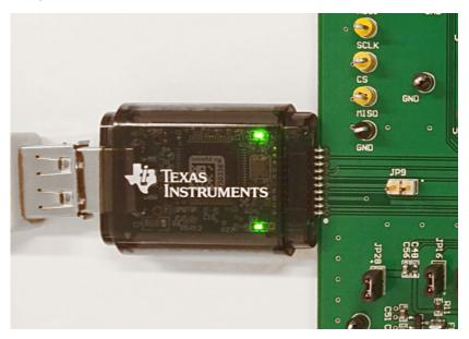
Figure 7. SM-USB-DIG Connection
