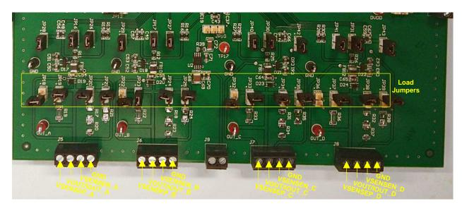
Figure 6. Output Terminal Block Connections and Load Jumpers
