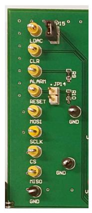
Figure 4. Digital Communication Test Points
