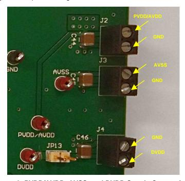
Figure 3. PVDD/AVDD, AVSS, and DVDD Supply Connections
