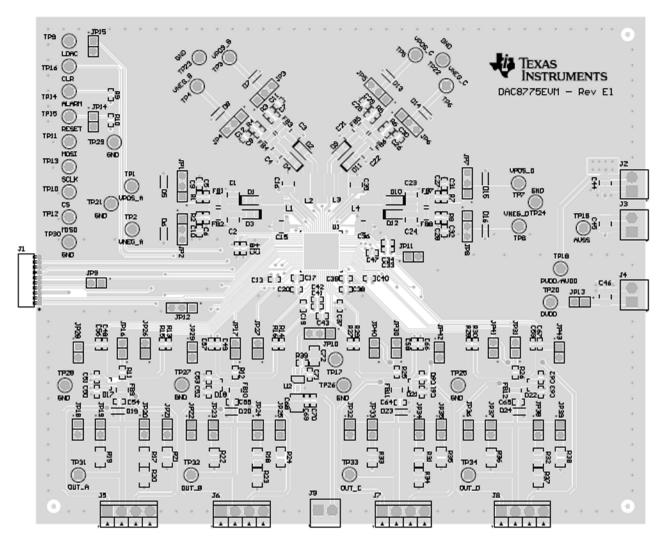
Figure 15. DAC8775EVM PCB Components Layout
