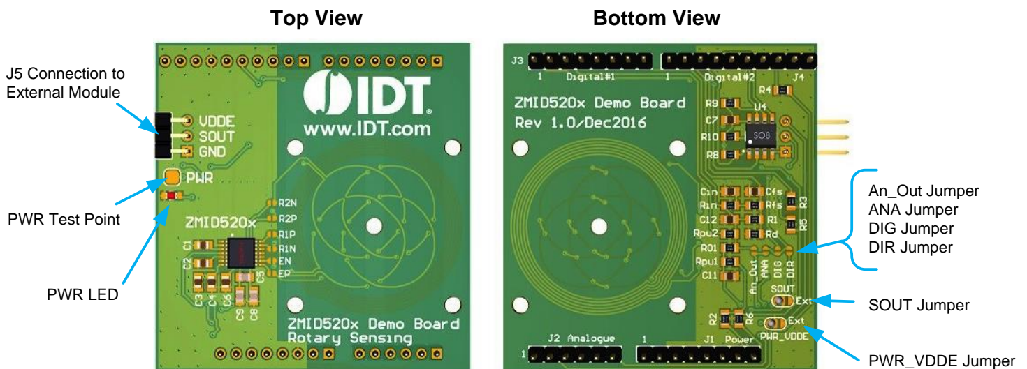
Figure 2. ZMID520x Rotary 360° Demo Board – Overview
