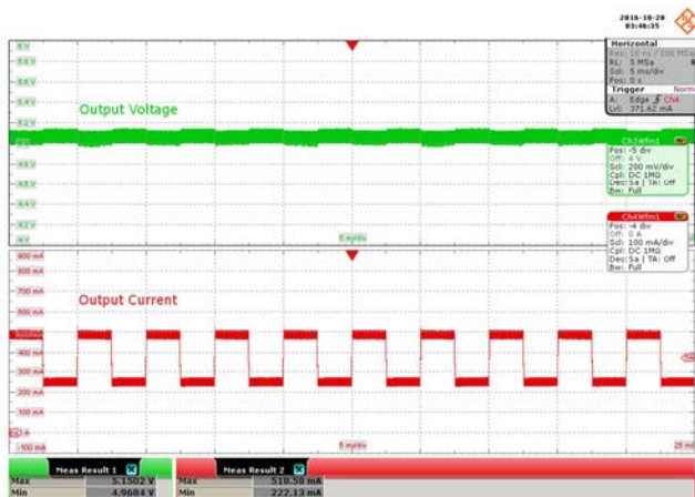
Figure 26 – 85 VAC Input. V_{OUT} , 200 mV / div. I_{OUT} , 100 mA / div., 5 ms / div. V_{MAX} : 5.1502 V. V_{MIN} : 4.9684 V.
