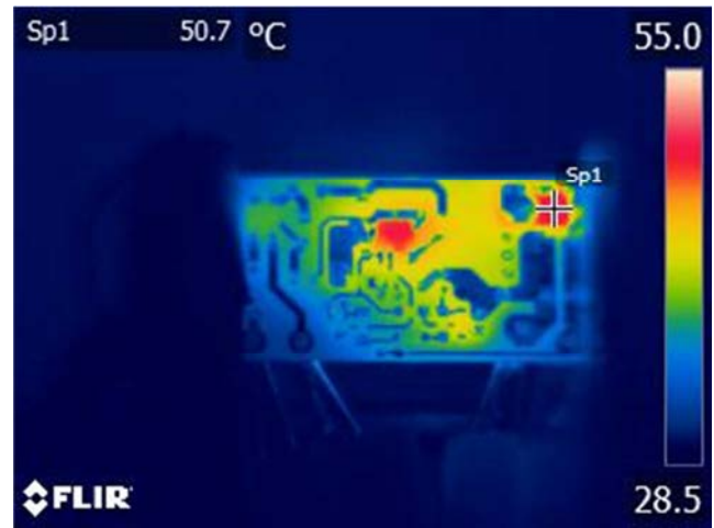
Figure 38 – Secondary Snubber Diode (D3). Spot: 50.7 °C.
