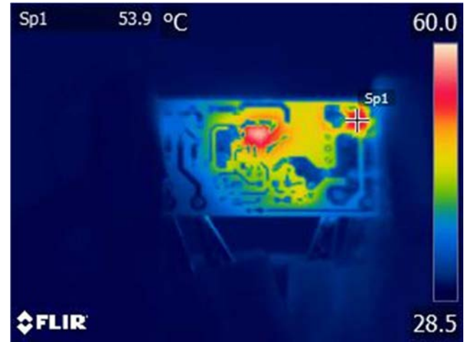
Figure 42 – Secondary Snubber Diode (D3). Spot: 53.9 °C.
