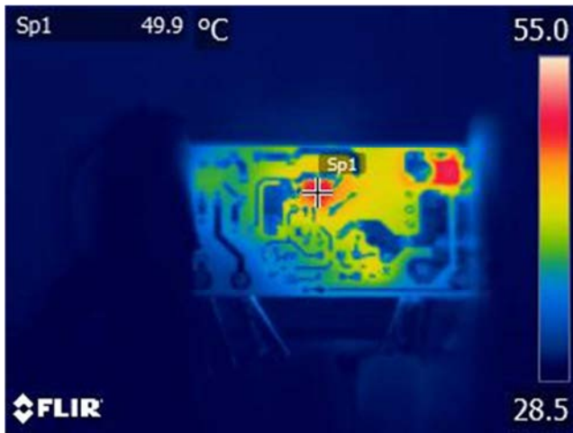
Figure 37 – LinkSwitch-XT2 (U1). Spot: 49.9 °C.
