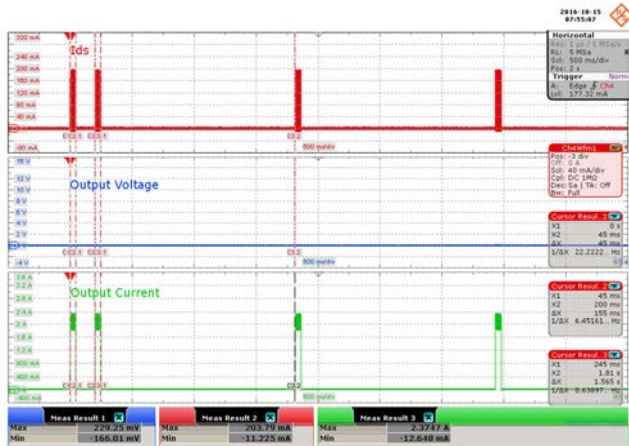
Figure 32 – 85 VAC Input. Condition: 5 V – Shorted. Upper: I_{DS} , 40 mA / div Middle: V_{OUT} , 2 V / div. Lower: I_{OUT} , 400 mA / div., 500 ms / div.
