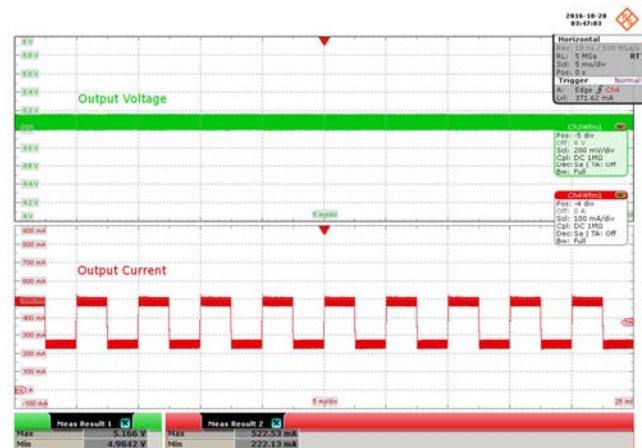
Figure 27 – 265 VAC Input. V_{OUT} , 200 mV / div. I_{OUT} , 100 mA / div., 5 ms / div. V_{MAX} : 5.166 V. V_{MIN} : 4.9842 V.
