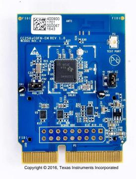
Figure 1. CC256xCQFN-EM Board
