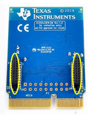
Figure 6. CC256XCQFN-EM Hardware Modifications for COM Connector
