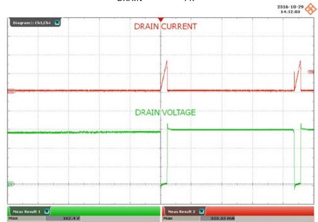
Figure 43 – 132 VAC, 60 V LED Load Upper: I_{DRAIN} , 200 mA / div. Lower: V_{DRAIN} , 50 V / div., 5 μs / div. Peak I_{DRAIN} : 325 mA PK . Peak V_{DRAIN} : 162 V PK .
