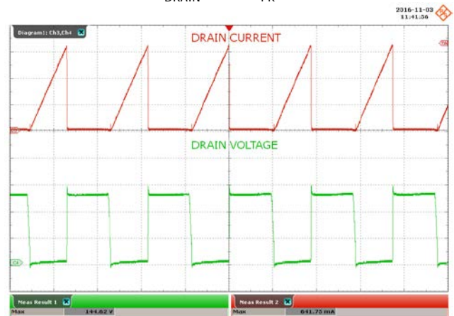
Figure 35 – 115 VAC, 60 V LED Load. Upper: I_{DRAIN} , 200 mA / div. Lower: V_{DRAIN} , 50 V / div., 5 \mu s / div. Peak I_{DRAIN} : 642 mA PK . Peak V_{DRAIN} : 144 V PK .
