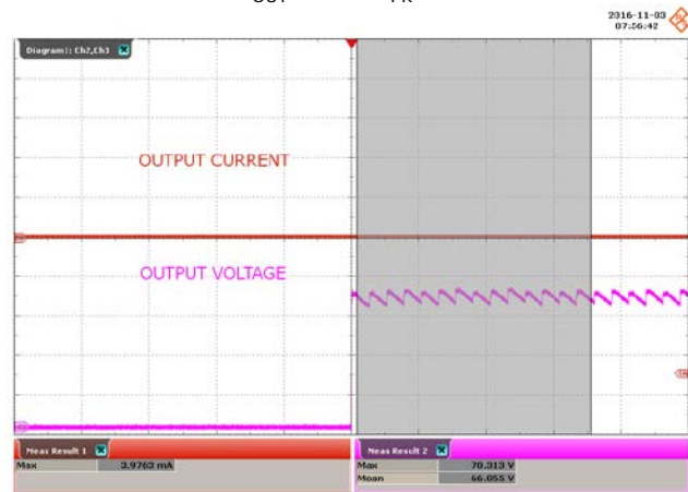
Figure 55 – 132 VAC, 60 V LED Load, Open Load Start-up. Upper: I OUT , 50 mA / div. Lower: V OUT , 20 V / div., 500 ms / div. Peak V OUT : 70.3 V PK .
