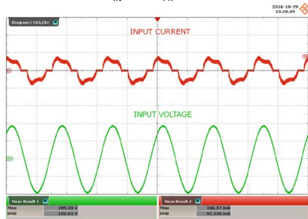
Figure 23 – 132 VAC, 60 V LED Load. Upper: I_{IN} , 200 mA / div. Lower: V_{IN} , 100 V / div., 10 ms / div. Peak I_{IN} : 167 mA PK . Peak V_{IN} : 189 V PK .
