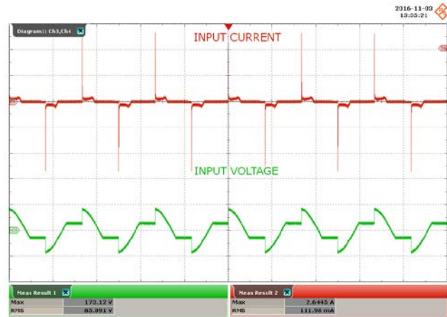
Figure 61 – 90° Conduction Angle. Upper: I_{IN} , 1 A / div. Lower: V_{IN} , 100 V / div., 10 ms / div. Peak V_{IN} : 173 V PK . V_{RMS} : 86 V.
