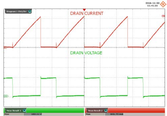
Figure 33 – 90 VAC, 60 V LED Load. Upper: I_{DRAIN} , 200 mA / div. Lower: V_{DRAIN} , 50 V / div., 5 \mu s / div. Peak I_{DRAIN} : 642 mA PK . Peak V_{DRAIN} : 103 V PK .
