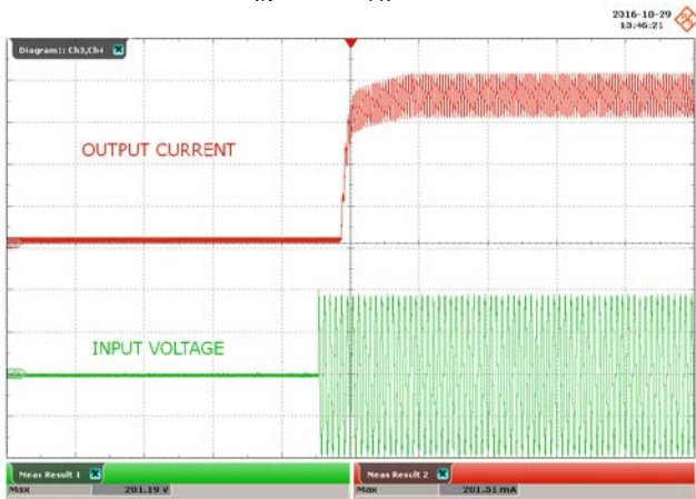
Figure 30 – 132 VAC, 60 V LED Load, Output Rise. Upper: I_{OUT} , 50 mA / div. Lower: V_{IN} , 100 V / div., 200 ms / div. Peak I_{OUT} : 202 mA PK . Peak V_{IN} : 201 V PK .
