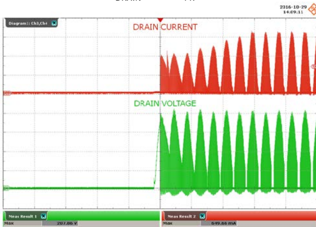
Figure 42 – 132 VAC, 60 V LED Load Upper: I_{DRAIN} , 200 mA / div. Lower: V_{DRAIN} , 50 V / div., 20 ms / div. Peak I_{DRAIN} : 650 mA PK . Peak V_{DRAIN} : 208 V PK .
