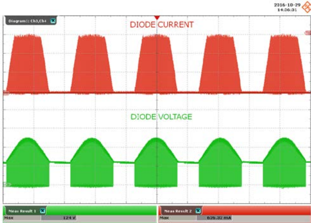
Figure 48 – 90 VAC, 60 V LED Load. Upper: I_{D3} , 200 mA / div. Lower: V_{D3} , 50 V / div., 4 ms / div. Peak I_{D3} : 626 mA PK . Peak V_{D3} : 124 V PK .
