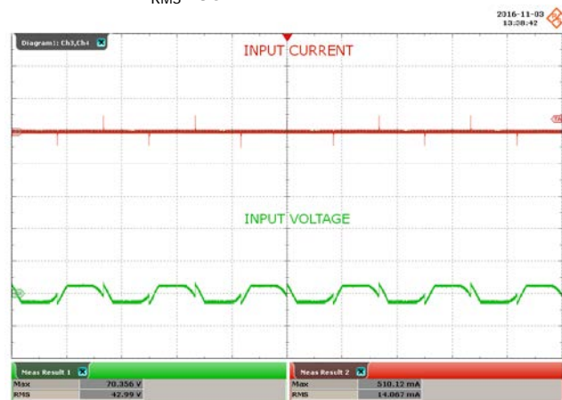
Figure 63 – 45° Conduction Angle. Upper: I_{IN} , 1 A / div. Lower: V_{IN} , 100 V / div., 10 ms / div. Peak V_{IN} : 70 V PK . V_{RMS} : 43 V.
