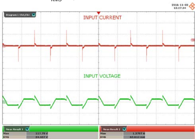
Figure 62 – 60° Conduction Angle. Upper: I_{IN} , 1 A / div. Lower: V_{IN} , 100 V / div., 10 ms / div. Peak V_{IN} : 118 V PK . V_{RMS} : 54 V.
