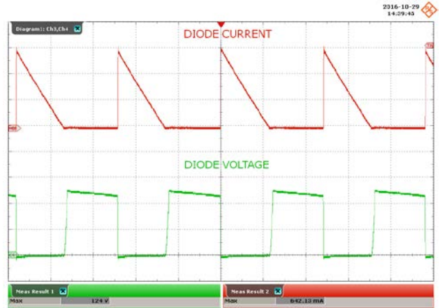
Figure 49 – 90 VAC, 60 V LED Load. Upper: I_{D3} , 200 mA / div. Lower: V_{D3} , 50 V / div., 4 \mu s / div. Peak I_{D3} : 642 mA PK . Peak V_{D3} : 124 V PK .
