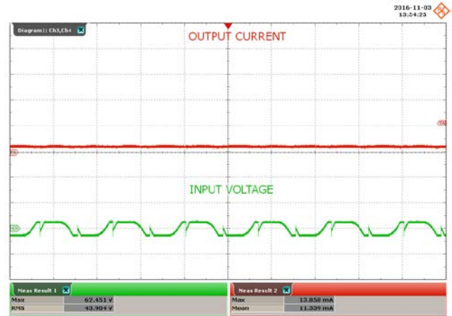
Figure 67 – 45° Conduction Angle. Upper: I_{OUT} , 50 mA / div. Lower: V_{IN} , 100 V / div., 10 ms / div. Peak I_{OUT} : 14 mA PK . Peak V_{IN} : 62 V PK .
