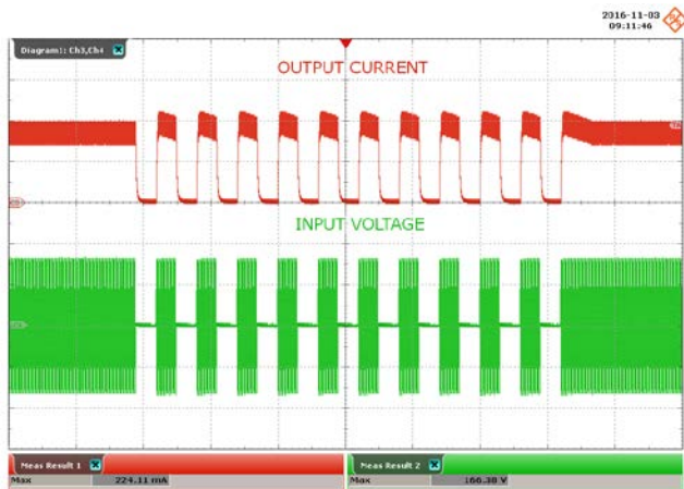
Figure 70 – 115 VAC, 60 V LED Load. 0.3 s On – 0.3 s Off. Upper: I_{OUT} , 100 mA / div. Lower: V_{IN} , 100 V / div., 1 s / div.
