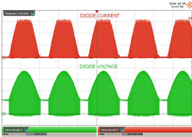
Figure 48 – 90 VAC, 60 V LED Load. Upper: I_{D3} , 200 mA / div. Lower: V_{D3} , 50 V / div., 4 ms / div. Peak I_{D3} : 626 mA PK . Peak V_{D3} : 124 V PK .
