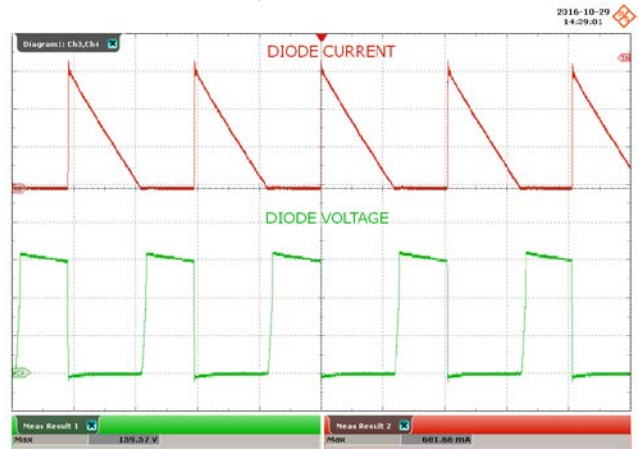
Figure 49 – 90 VAC, 60 V LED Load. Upper: I_{D3} , 200 mA / div. Lower: V_{D3} , 50 V / div., 4 \mu s / div. Peak I_{D3} : 642 mA PK . Peak V_{D3} : 124 V PK .
