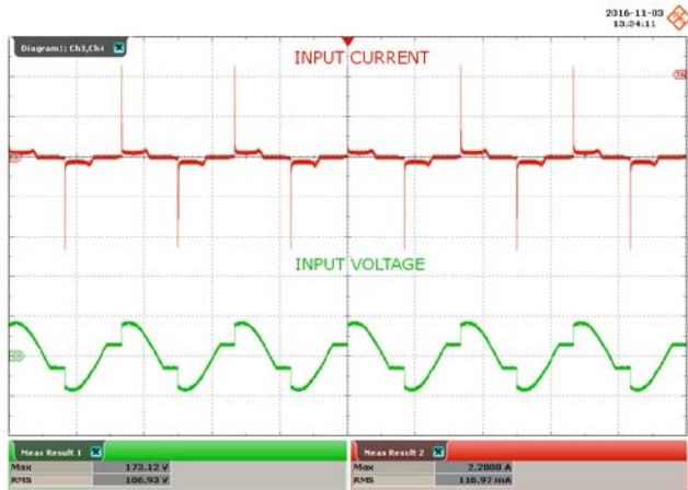
Figure 60 – 120° Conduction Angle. Upper: I_{IN} , 1 A / div. Lower: V_{IN} , 100 V / div., 10 ms / div. Peak V_{IN} : 173 V PK . V_{RMS} : 107 V.
