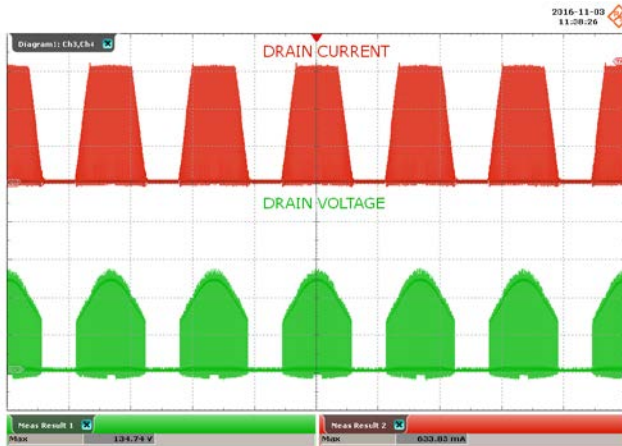
Figure 32 – 90 VAC, 60 V LED Load. Upper: I_{DRAIN} , 200 mA / div. Lower: V_{DRAIN} , 50 V / div., 5 ms / div. Peak I_{DRAIN} : 634 mA PK . Peak V_{DRAIN} : 135 V PK .
