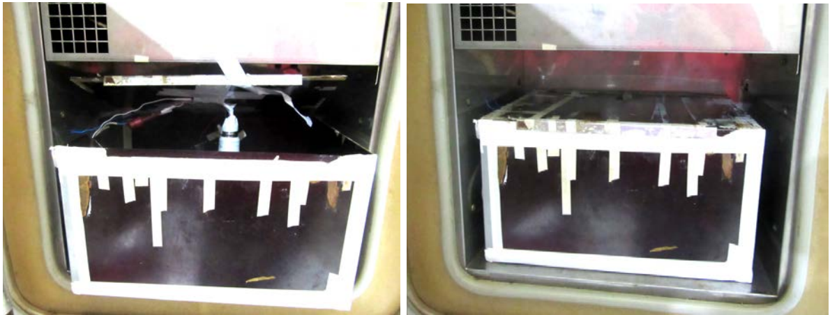
Figure 15 – Test Set-up Picture – Inside BR-30 Bulb Casing.
