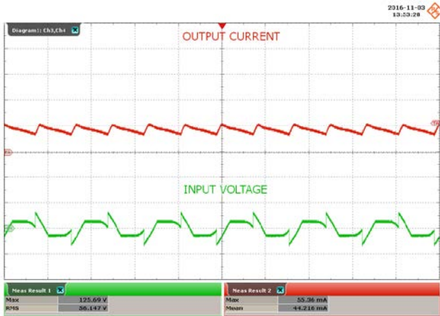
Figure 66 – 90° Conduction Angle. Upper: I_{OUT} , 50 mA / div. Lower: V_{IN} , 100 V / div., 10 ms / div. Peak I_{OUT} : 55 mA PK . Peak V_{IN} : 125 V PK .
