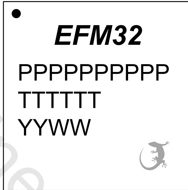
Figure 6.3. BGA192 Package Marking
