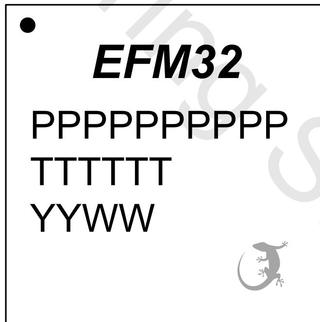
Figure 7.3. TQFP100 Package Marking
