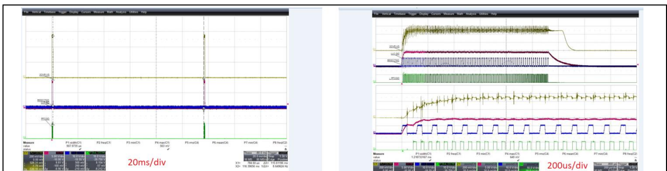
Figure 10 Typical waveforms during standby(left:20 ms/div; right: 20 ms/div)
