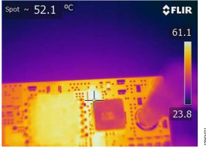
Figure 30. Thermal Image of SR1 at 48  $V_{DC}$  Input, 6 A Load, No Airflow, 1 Hour Soaking Time
