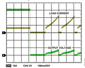
Figure 15. Over Current Protection (OCP) under Output Short Circuit at 48 V DC Input; the Under Voltage Lockout Threshold of the VDD2 Pin (VDD2\_UVLO) Causes the First hiccup time of ~200 ms and the OCP Causes the Subsequent Hiccup Time of ~40 ms
