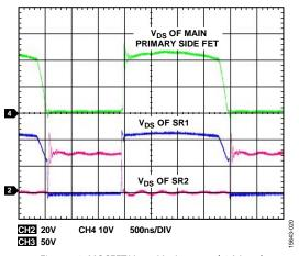
Figure 19. MOSFET V<sub>DS</sub> at V<sub>DC</sub> Input and 6 A Load
