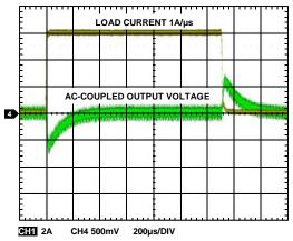
Figure 11. Transient Response with Load Steps, 0% to 100%
