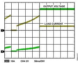
Figure 16. Recovery from Output Short Circuit at 48 V<sub>DC</sub> and 6 A Load
