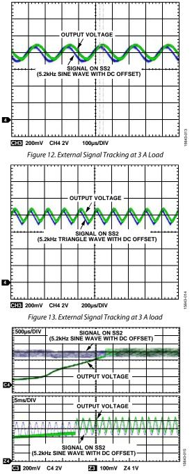
Figure 14. External Signal Tracking at 3 A Load During Start Up
