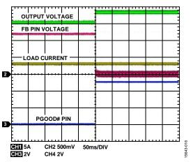
Figure 17. Overvoltage Protection (FB Pin Shorted to the ANGD2 pin)
