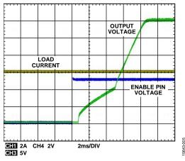
Figure 4. Soft Start at 48 V DC Input, 0 A Load
