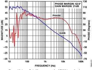
Figure 10. Loop Gain Measurement by AP200 Loop Analyzer; 48 V Input, 6 A Load, Crossover Frequency at 12.06 kHz Transient Response for Load Step
