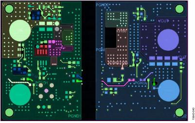
Figure 39. PCB Layout, Layer 4
