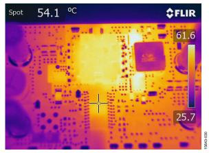
Figure 29. Thermal Image of ADP1074 at 48  $V_{\rm DC}$  Input, 6 A Load, No Airflow, 1 Hour Soaking Time
