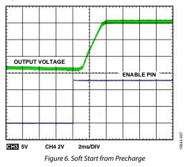
Change the slope of the first stage of soft start by changing the SS1 capacitor. Alternate soft start slopes can be selected by changing the SS1 capacitor.
