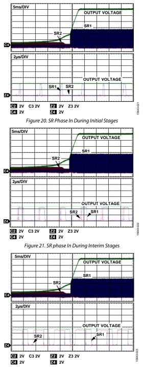
Figure 22. SR Phase In During Later Stages
