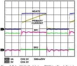
Figure 2. Pulse-Width Modulations (PWMs) at Steady State Load
