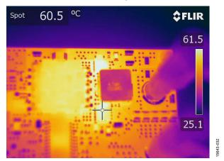
Figure 31. Thermal Image of SR2 at 48  $V_{\rm DC}$  Input, 6 A Load, No Airflow, 1 Hour Soaking Time
