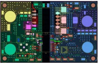
Figure 36. Printed Circuit Board (PCB) Layout, Top Layer
