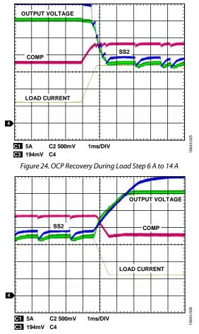
Figure 25. OCP Recovery During Load Dump, 14 A to 6 A
