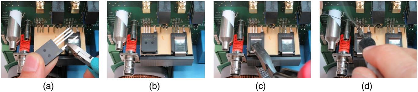
Figure 6 Assembling a device onto the heat sink and the PCB
