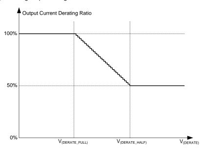
Figure 5. Output-Current Derating Profile
