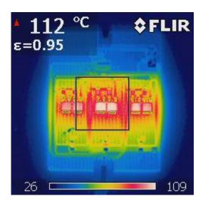
Figure 11. Thermal Image of DRL Function at 25°C, 12-V Input Voltage
