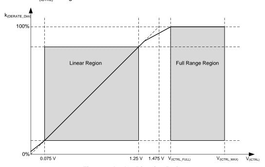
Figure 6. Analog Dimming Ratio
