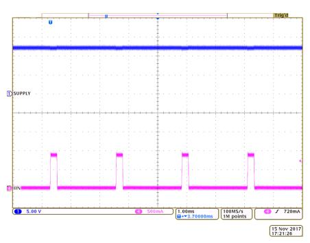
Figure 10. Position Light Function Waveform—CH1: Supply Voltage, CH4: Input Current
