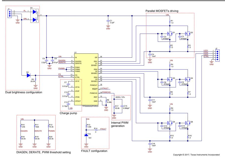
Figure 2. TIDA-01375 Schematic
