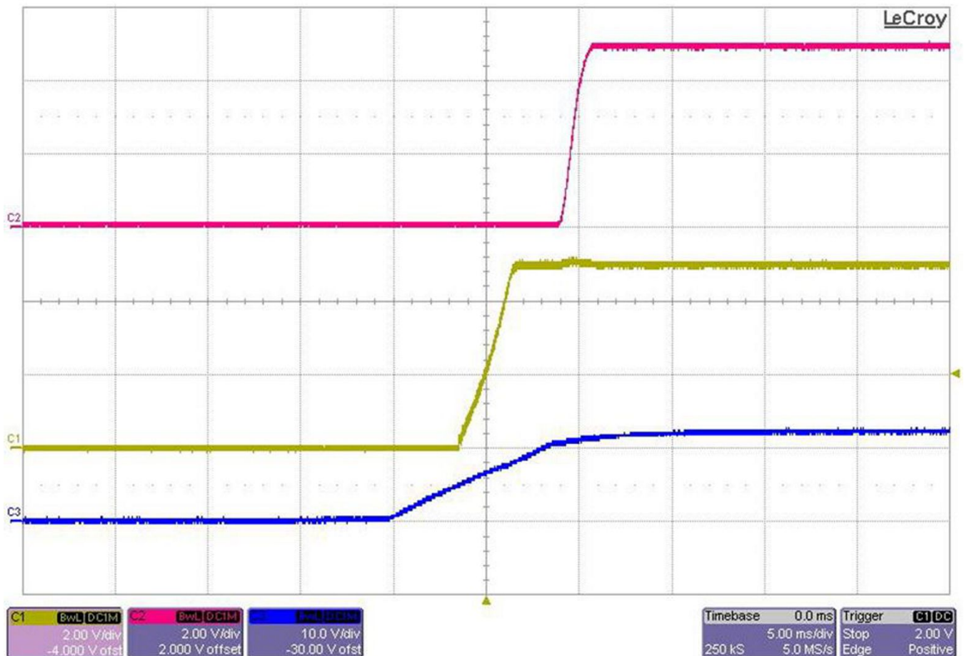
Figure 5. Start-Up Waveform: Vin = 12 V, Vout = 5 V, Iload = 0 A
