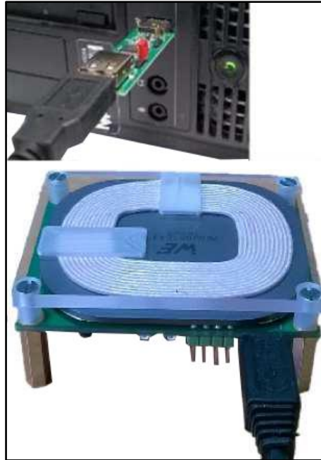
Figure 14: USB-to-UART dongle to STEVAL-ISB044V1 connection
