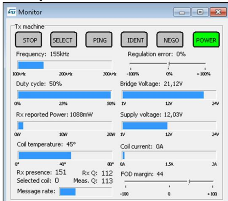
Figure 35: STSW-STWBCGUI: Qi monitor window
