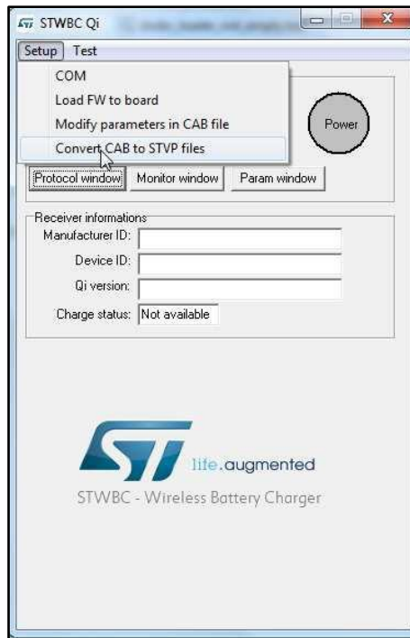
Figure 24: STSW-STWBCGUI: convert CAB to STVP files
