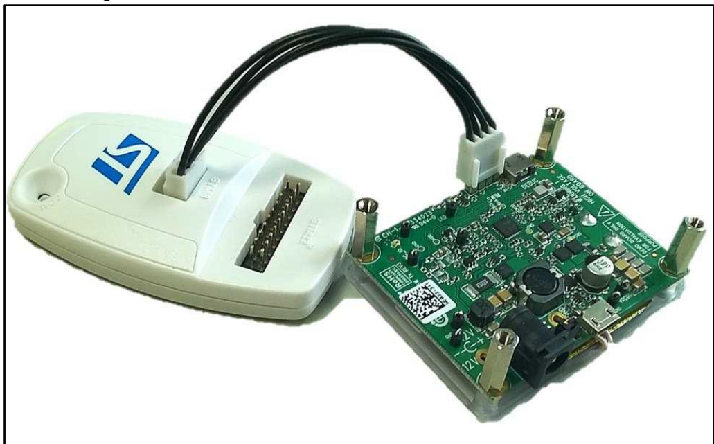
Figure 17: STEVAL-ISB044V1 evaluation board: ST-LINK connection
