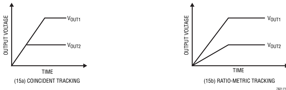
Figure 15. Two Different Methods of Output Voltage Tracking
