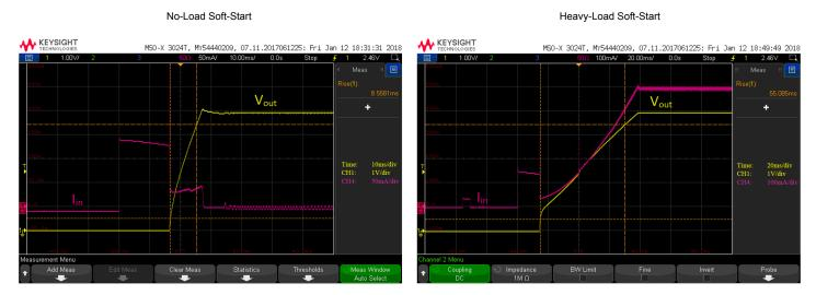
Figure 8.1. Si34061 Isolated Flyback C4 EVB Input Current and Output Voltage Soft-Start at Low Load (Left) and Heavy Load (Right) Conditions
