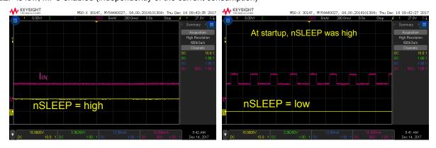
Figure 14.2. With nSLEEP High, MPS is Disabled (Left); with nSLEEP Low, MPS is Enabled (Right); MPS
