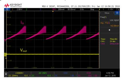
Figure 9.1. Si34061-Isolated Flyback C4 EVB Output Voltage and Input Current when Output is Shorted
