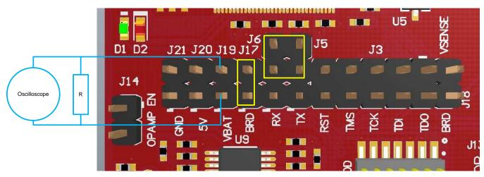
Figure 17. Active Power Measurements (>1 mA)
