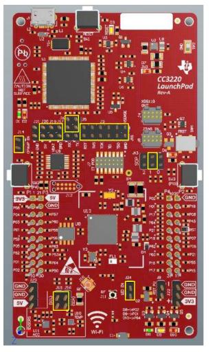
Figure 13. Powering From USB Jumper Settings
