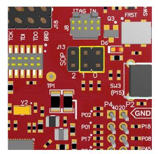
Figure 9. SOP Jumpers (Default Setting Shown)
