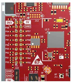
Figure 4. Pin 1 Marking on CC3220LP (3V3 Tag)
