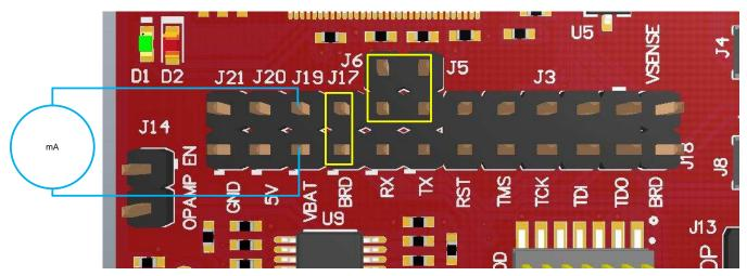
Figure 16. Low-Current Measurement (<1 mA)
