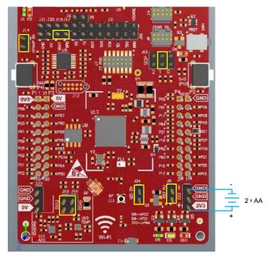
Figure 14. Powering the CC3220LP From Battery
