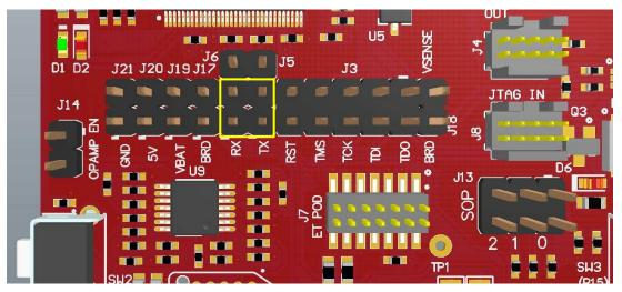
Figure 11. UART Routed to 20-Pin Header Connector
