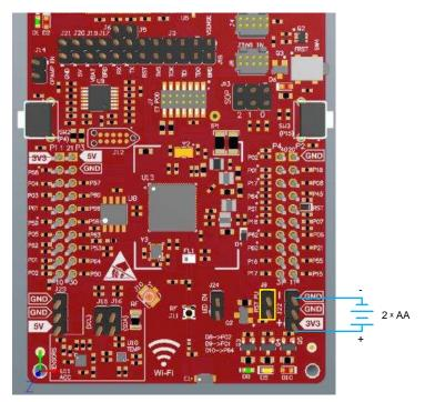
Figure 15. Only CC3220 and Serial Flash Powered by Battery
