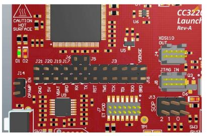
Figure 5. Default Jumper Configuration for JTAG Lines
