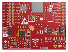
Figure 7. I<sup>2</sup>C Bus Connections
