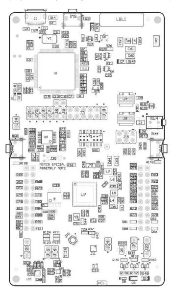
Figure 20. CC3220x LaunchPad Top-Layer Assembly Drawing
