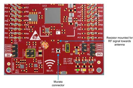
Figure 18. Using Onboard Antenna (Default Condition)
