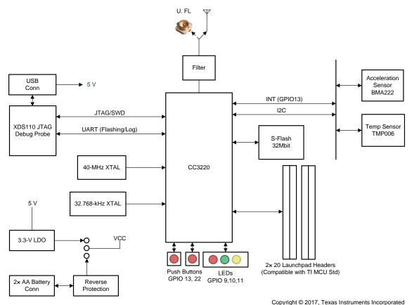
Figure 3. CC3220 Block Diagram
