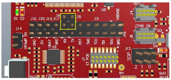
Figure 10. UART Routed to USB COM Port
