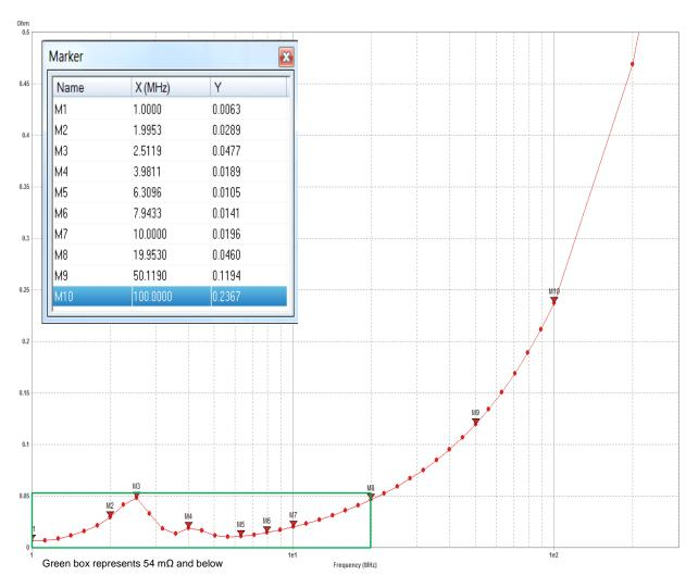
Figure 19. Target Impedance: VDD\_DSP\_AVS
