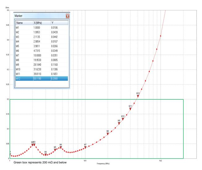
Figure 23. Target Impedance: VDD\_DDR\_1V35
