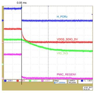
Figure 12. TPS65919 Stage One Power Down
