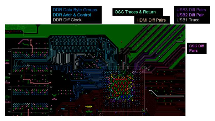
Figure 4. High-Speed Signaling Breakout Overview(Top)
