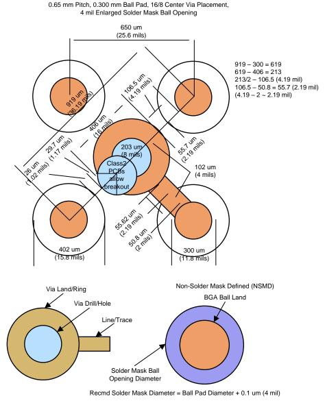
Figure 2. 16/8 Center Via Placement Breakout Scheme
