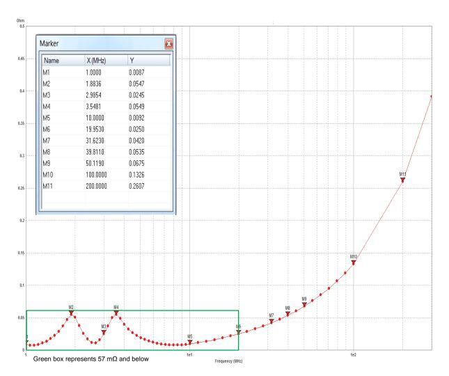
Figure 21. Target Impedance: VDD\_CORE\_AVS
