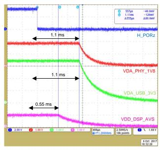
Figure 14. TPS65919 Stage Two and Three Power Down
