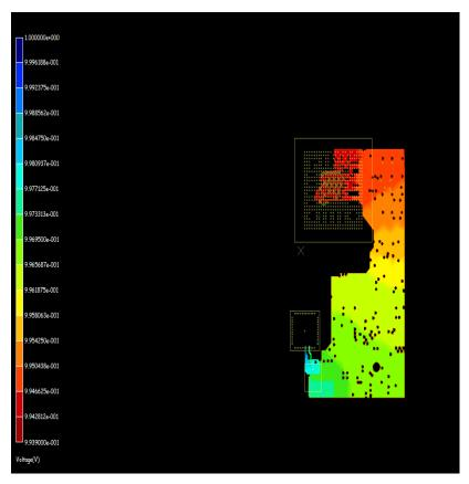
Figure 20. VDD\_CORE\_AVS IR Drop Analysis
