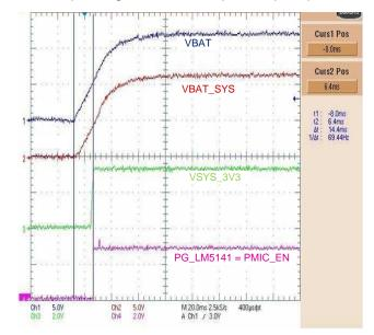
This appendix shows oscilloscope images of the initial power up sequence of the TPS65919 PMIC.
