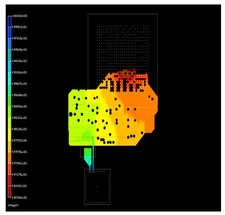
Figure 18. VDD\_DSP\_AVS IR Drop Analysis
