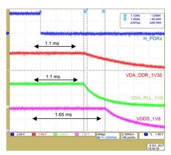
Figure 16. TPS65919 Stage Three and Four Power Down
