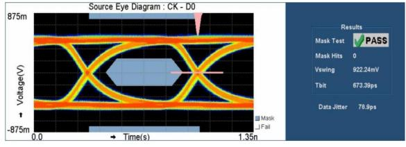
Figure 5. HDMI Eye Diagram Waveform
