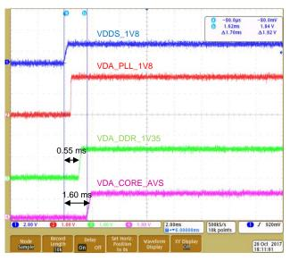
Figure 8. TPS65919 Stages Four and Five Power Up
