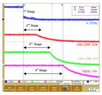
Figure 17. TPS65919 All Four Stages Power Down
