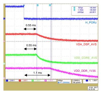
Figure 15. TPS65919 Stage Two and Three Power Down (Continued)
