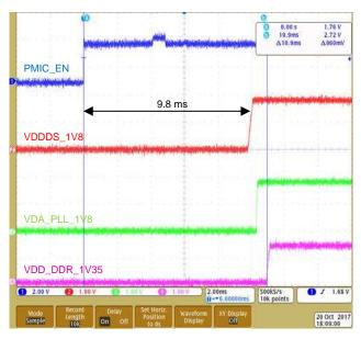
Figure 7. TPS65919 Stages One to Three Power Up
