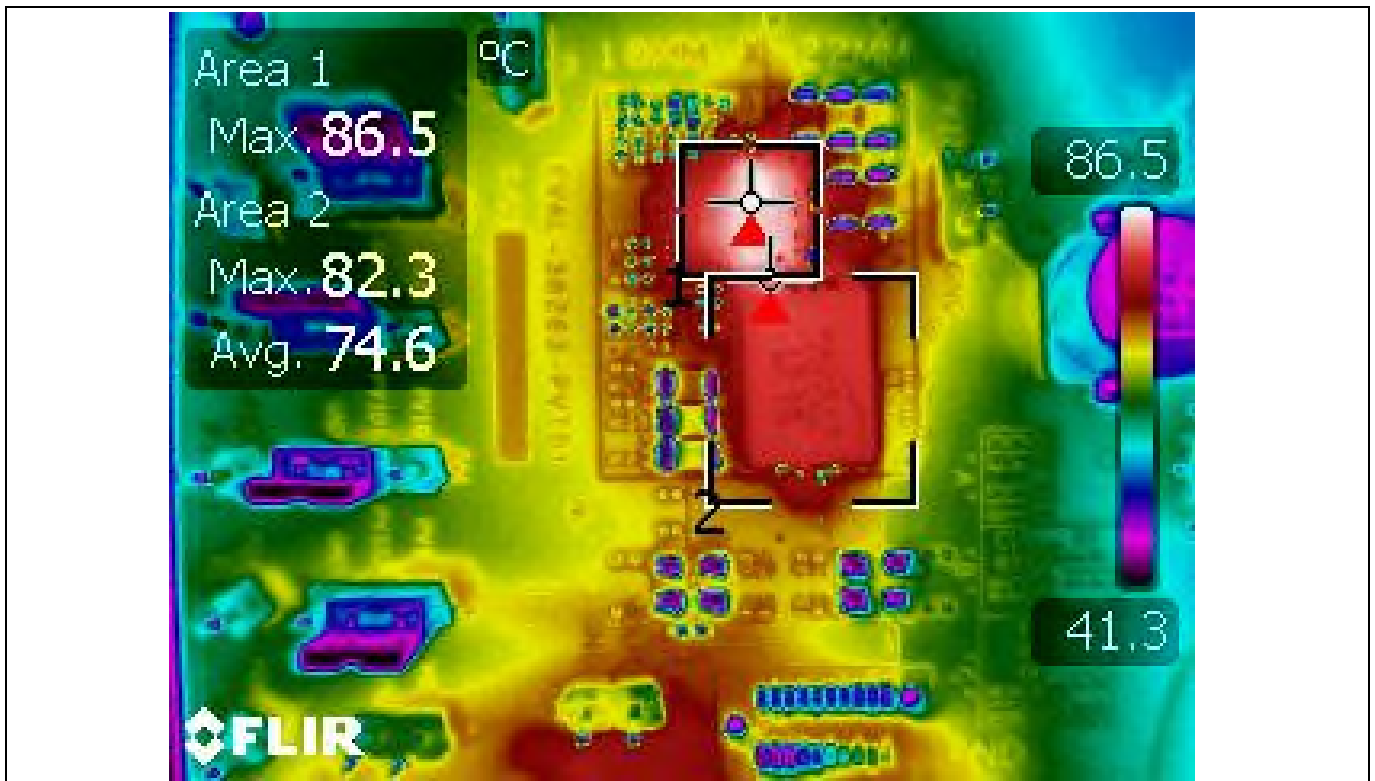
Figure 33 Thermal Image of the board at 30 A load, IR38263: 86.5°C, inductor: 82.3°C
