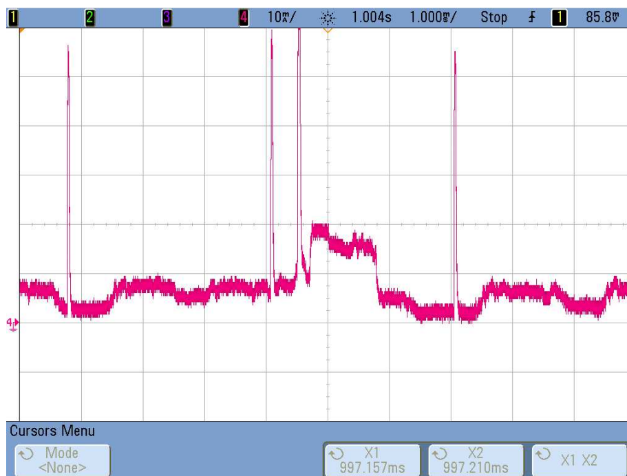
Figure 59. Pulse Showing Standard BLE Once Connected
