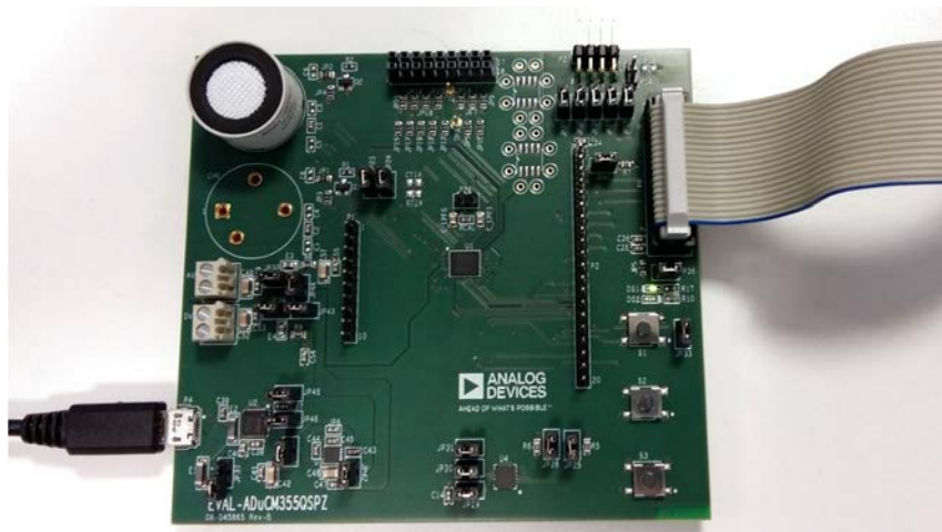
Figure 2. Power via Micro-USB Cable Directly
