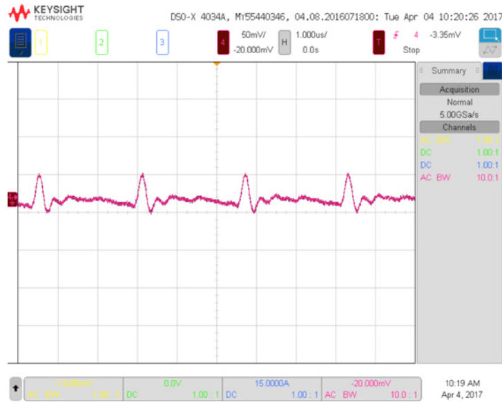
Figure 5. Output Ripple at 100V_{IN} , 5V_{OUT} and 2.3A_{OUT} (50mV, 500ns/DIV, 20MHz Bandwidth)
