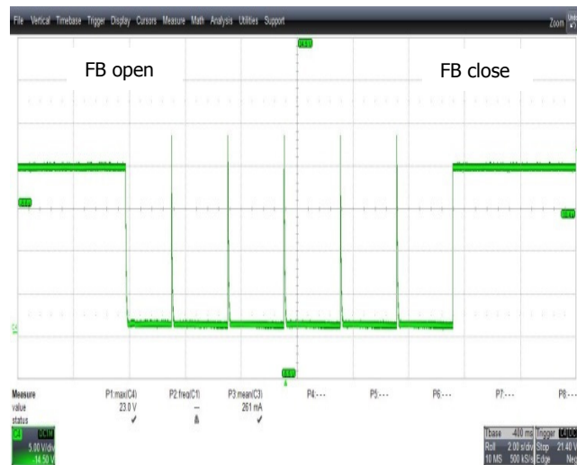
Figure 40 – Output Voltage Waveform. 90 VAC Input. (OVP = 23 V.) V OUT : 5 V, 2 s / div..
