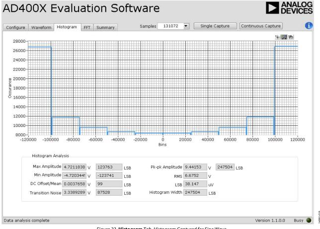
Figure 22. Histogram Tab, Histogram Captured for Sine Wave
