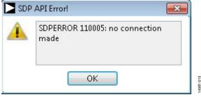
Figure 16. SDP-H1 Board Not Connected to the USB Port Error
