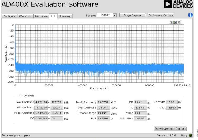
Figure 23. FFT Tab (AD4003 Running in Turbo Mode)
