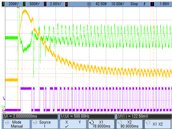
Figure 24. Upward Motor Operation at 12 V With 60 Pounds of Added Weight
