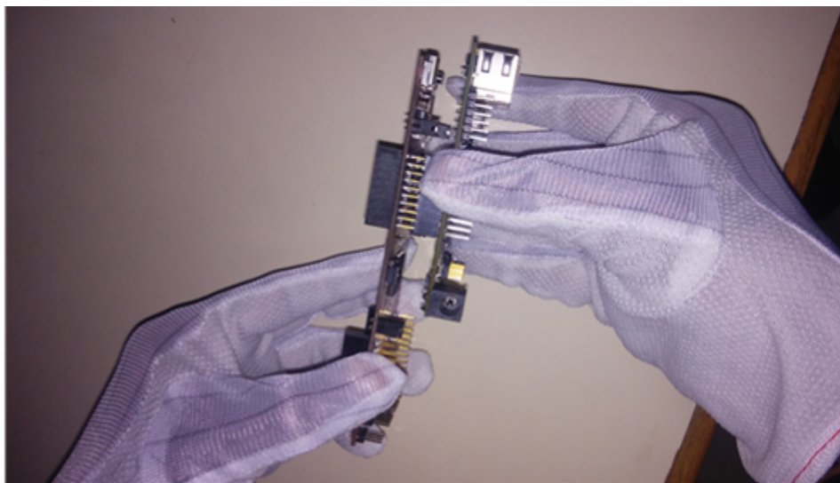
Figure 23. AMIC110 ICE and F28069M LaunchPad Connection (2 of 2)
