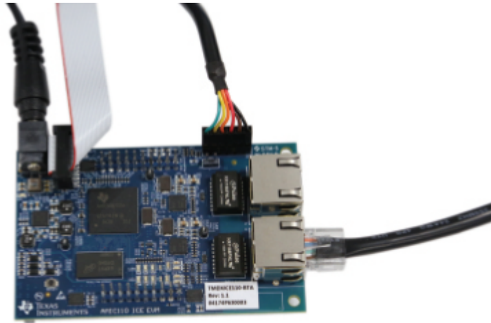
Figure 4. AMIC110 ICE Power Supply Connection
